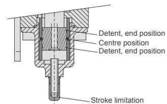
**Fig. 21 Friction brake / detent**
