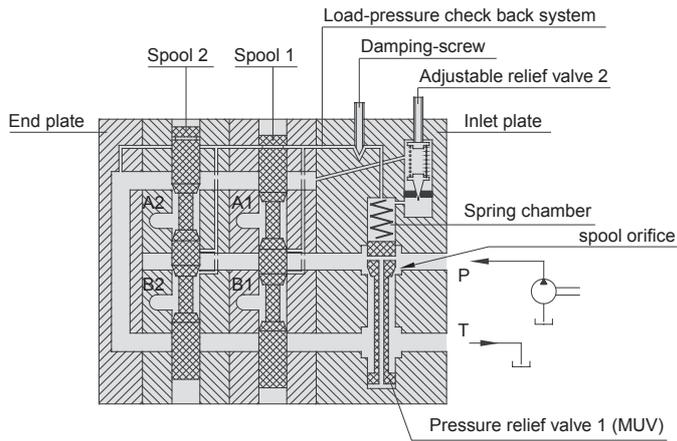
**Fig. 7 By-pass flow control valve**
