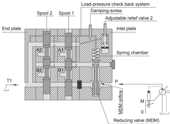
**Fig. 9 Series flow control valve**
