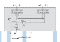
Fig. 11 By-pass flow control valve
