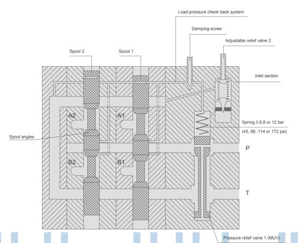
Free recirculation pressure P—→T MUV with 3, 6, 8 or 12 bar spring (43, 86, 114 or 172 psi).
