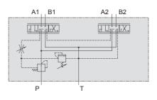
Fig. 9 Series flow control valve
