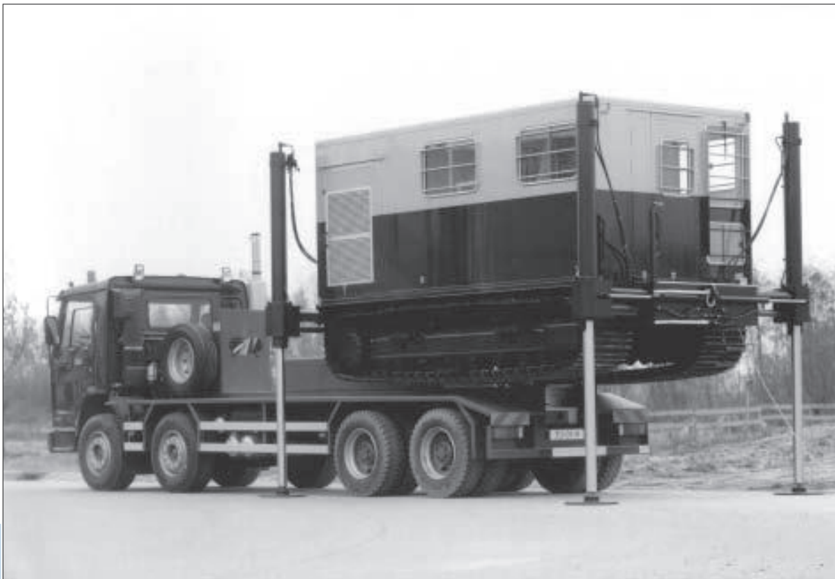
Fig. 20 Cone Penetration Testing Unit, The Netherlands
